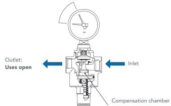
When the uses to be served are closed, the downstream pressure increases, pushing the reducer piston downwards. In this way, the shutter closes the passage section of the reducer maintaining the setting value set on the spring constant; in fact, the minimum pressure difference across the shutter permits the perfect closing of this latter.
