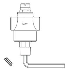
The final calibration of the pressure reducing valve must be performed with the hydraulic circuit completely full and with all the uses closed, otherwise false values would be obtained owing to the fact that the downstream pressure reduces in relation to the necessary flow rate, during any supply.
